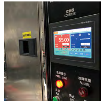
Full-load operation at an ambient temperature of 55°C.
