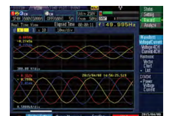
Voltage and current of spot welding machine after treatment
