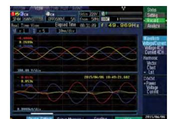
Voltage and current of spot welding machine before treatment
